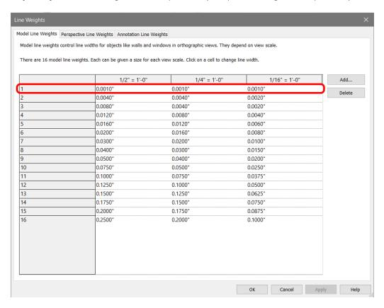
If you change the line weight assigned to Pen #1 you will change the line weight of ALL your surface patterns. (found on Revit Manage Ribbon -> Additional Settings -> Line Weights) Because of this behavior, we recommend reserving Pen 1 for surface patterns only, and not using it for any other geometry or line work. (Give us a ring if you would like to have that discussion.)
