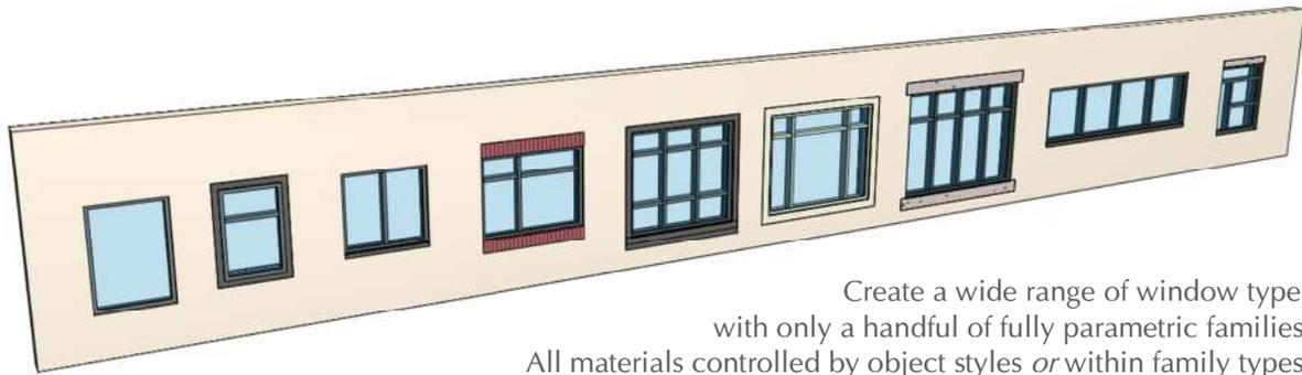
Create a wide range of window types with only a handful of fully parametric families. All materials controlled by object styles *or* within family types.
